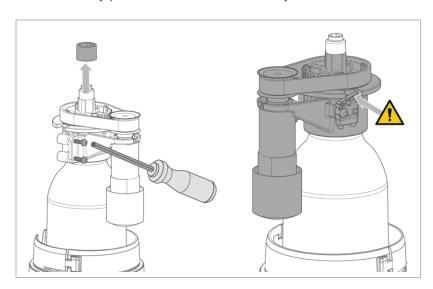
10. Check the motor unit for wear and tear.
