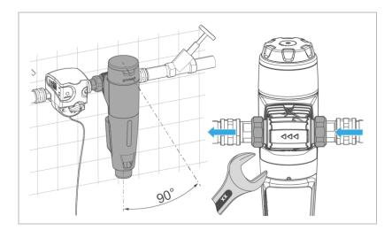
**5.** Tighten the click-type connection flange with the union nuts without applying any mechanical stress.
