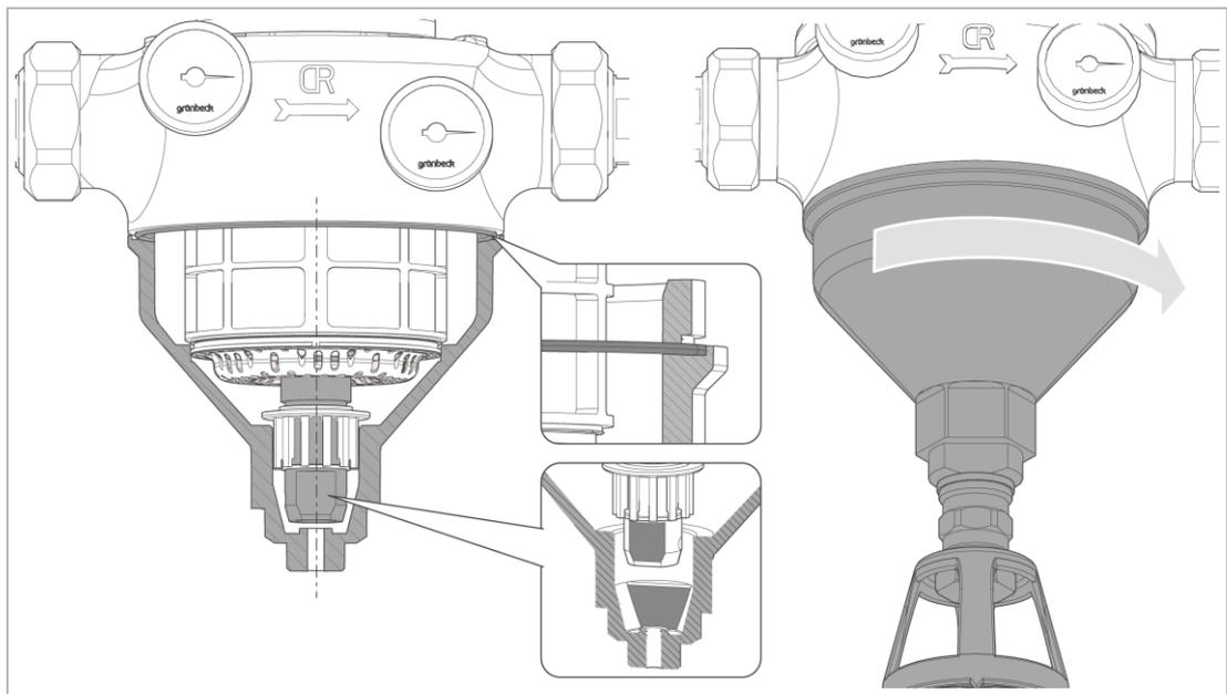
5. Screw the filter funnel onto the filter housing.
