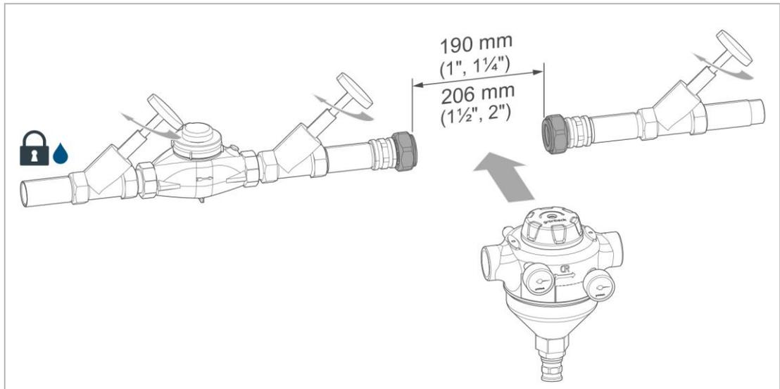
1. Install the water meter screw connection in the pipe.
