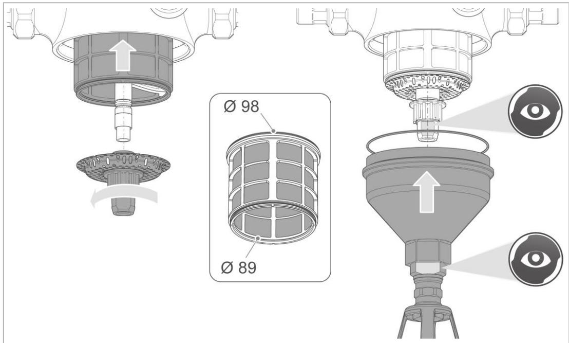
1. Fit the O-rings to the filter elements. Slide the filter elements with the larger  $\varnothing$  pointing forward over the suction nozzle into the filter housing.
