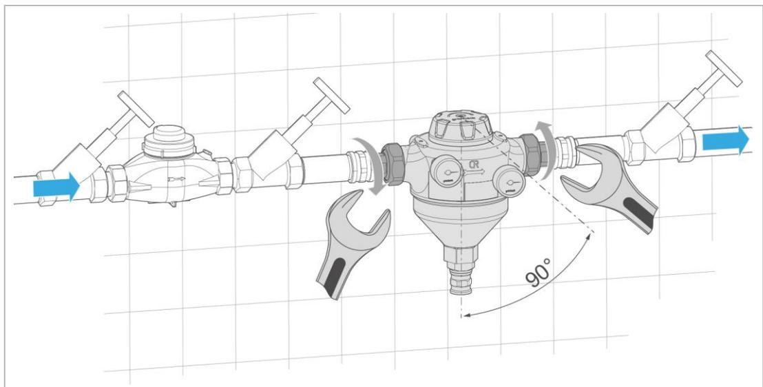
3. Install the filter without stress and tighten the union nuts.
