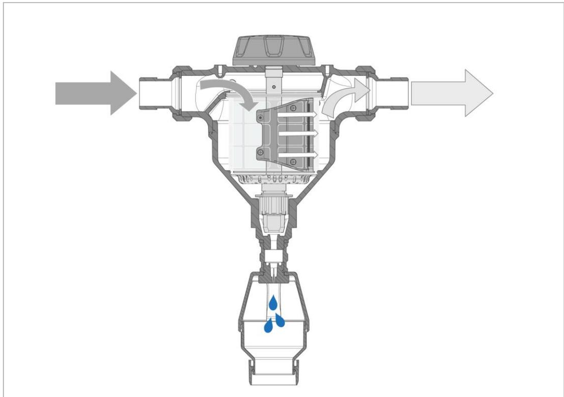
The unfiltered raw water flows into the filter from the inlet side and from the inside out through the filter element and to the pure water outlet. Thus, foreign particles of  $> 100 \mu\text{m}$  in size are retained.
