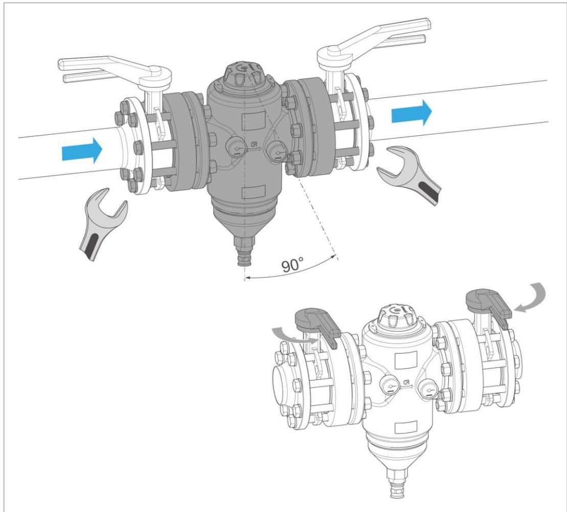
2. Position the filter in the pipe.
