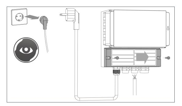
▶ Unscrew the cover of the connections at the control unit.
