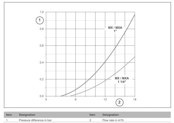
Pressure loss curves of GENO-backwash filters MXA 1" and 11/4"
