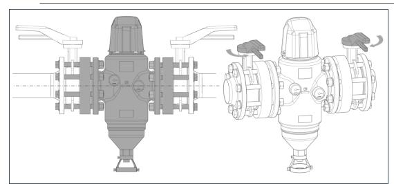
• Check the function of the shut-off valves after installation.
