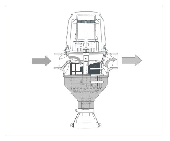
The unfiltered raw water flows into the filter from the inlet side and then from the inside out through the filter element and to the pure water outlet.
