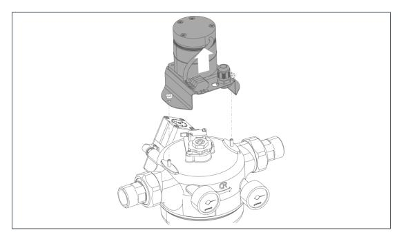
6. Lift the motor unit off the filter housing.
