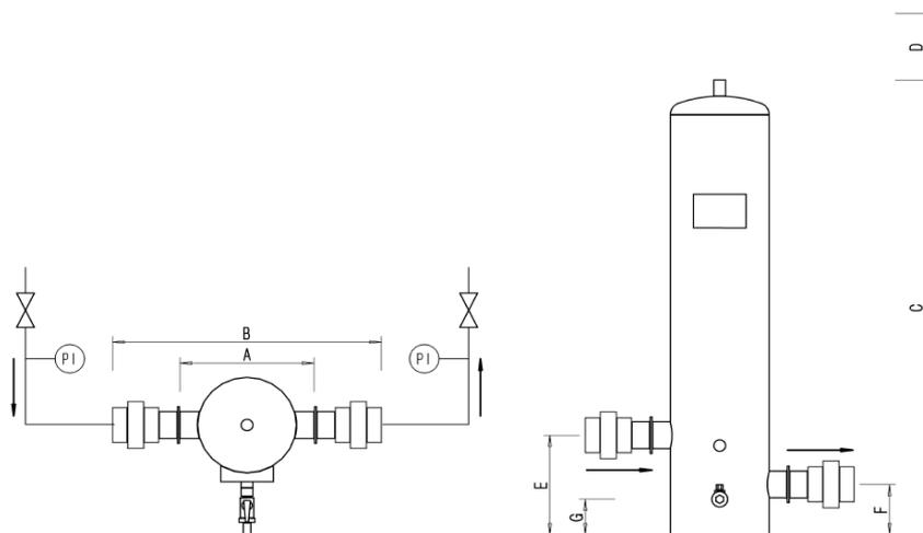
Fig. 4: Installation/dimensional drawing of a GENO-activated carbon filter AKF 1600/6000
