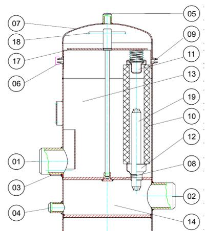
Fig. 3 Exploded drawing of a GENO-activated carbon filter AKF
