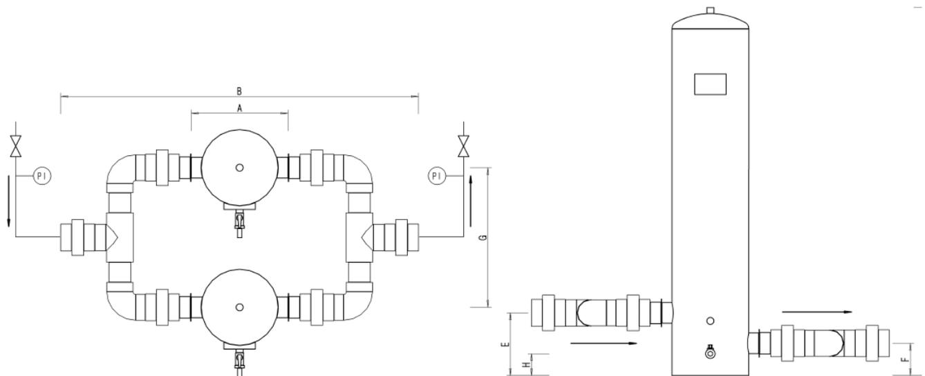
Fig. 5: Installation/dimensional drawing of a GENO-activated carbon filter AKF 9000/12000
